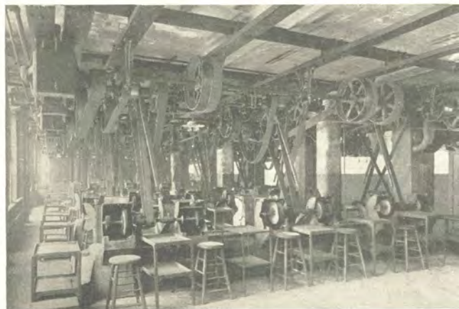
Fig. 3—What the Average Belt-Driven Buffing Equipment Looks Like
